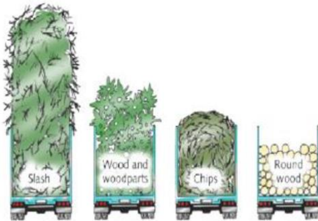
Illustration ; Energy Density Differences of the same Weight Material by Different Product
